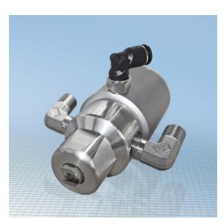
Pneumatic operated valve for automated airless applications. The valve body is made of stainless steel in the fluid section and aluminum in the pneumatic drive. This makes KS-AKA 421 suitable for solvent and water based materials.
