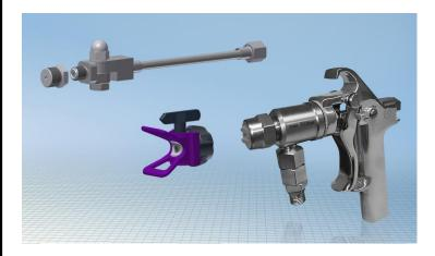
Another useful accessory for the KS1 (L) is the reverse tip adapter. Besides of the standard airless flat spray nozzles a reverse tip nozzles can be used alternatively. These nozzles are rotatable at 180° without dismounting. When a tip clog occurs, turn the tip from spray to clean position and pull the trigger for quick a burst of fluid flow. This action will clean the orifice of the particle causing the tip clog. Reverse tip nozzles are also available with an integrated preatomizer.
