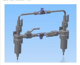
Twin filter unit with two 3/2 ways ball valves for switching between the filter lines. This very compact option uses only little mounting space. The material input of the unit is from the bottom and the outlet is at the top ball valve. The basic version of the unit has an internal 3/8" thread which can be equipped with different nipples or connectors as required by the application.
