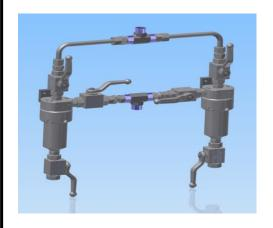
Twin filter unit with four 2/2-ways ball valves for switching between the filter lines. This option is the most cost effective twin filter unit in stainless steel. The material input of the unit is from the bottom and the outlet is at the top T-fitting. The basic version of the unit has an internal 3/8" thread which can be equipped with different nipples or connectors as required by the application.
